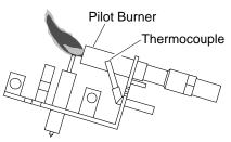
Figure 24 - Incorrect Pilot Flame Pattern
